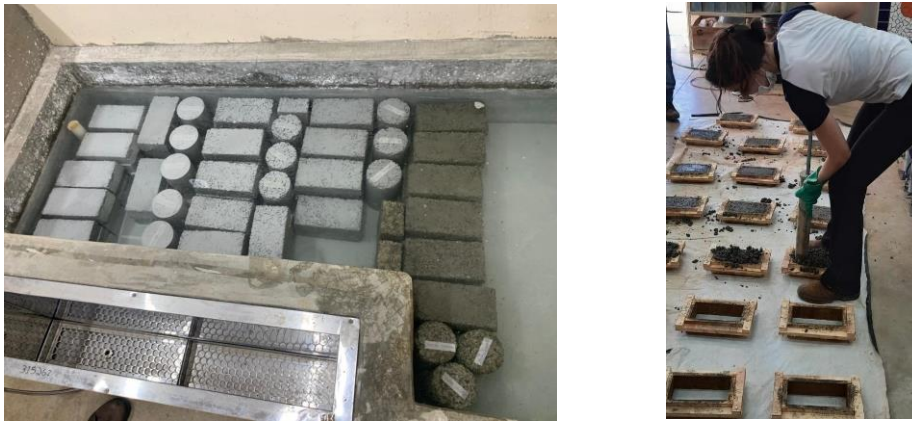
FIGURE 2. The casting of concrete blocks (left) and immersion curing (right).
