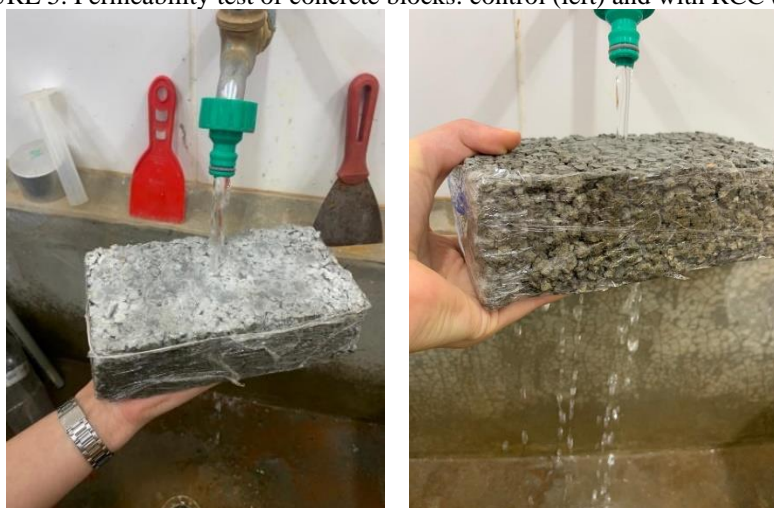
FIGURE 5. Permeability test of concrete blocks: control (left) and with RCC (right) .
