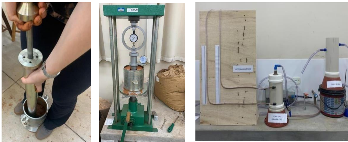
FIGURE 1. Soil tests: compaction (left), CBR (center) and permeability (right).
