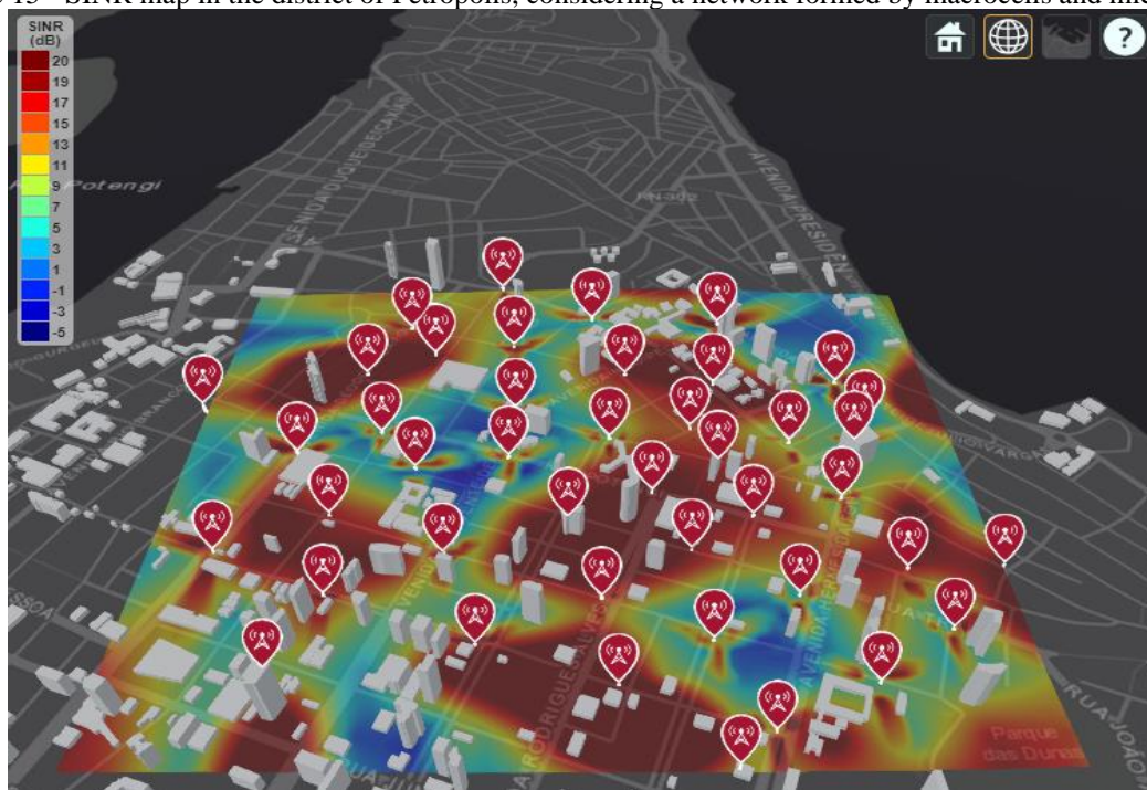
Figure 15 - SINR map in the district of Petrópolis, considering a network formed by macrocells and microcells.
