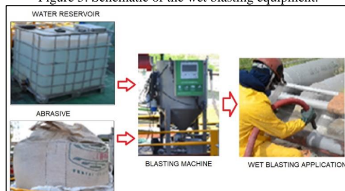
Figure 5: Schematic of the wet blasting equipment.
