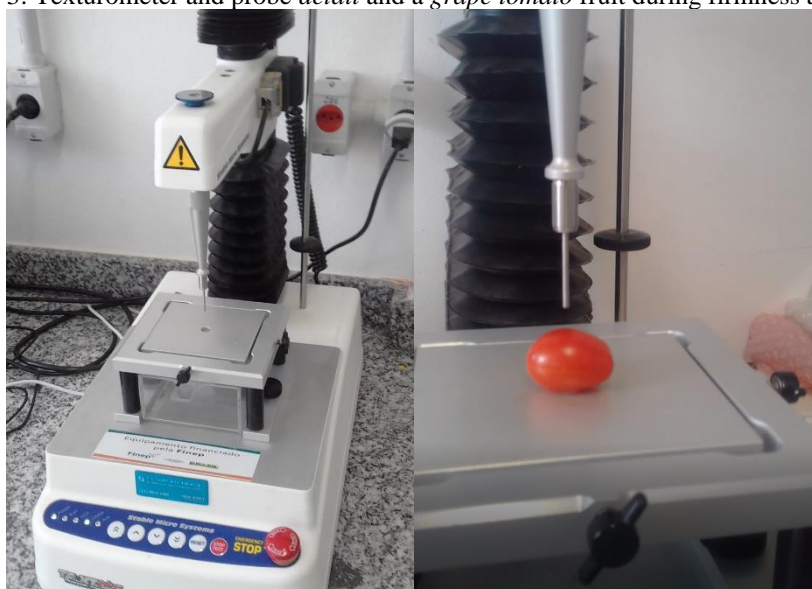
Figure 3: Texturometer and probe detail and a grape tomato fruit during firmness analysis.
