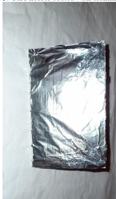
Figure 3: Card holder coated with aluminum foil.
