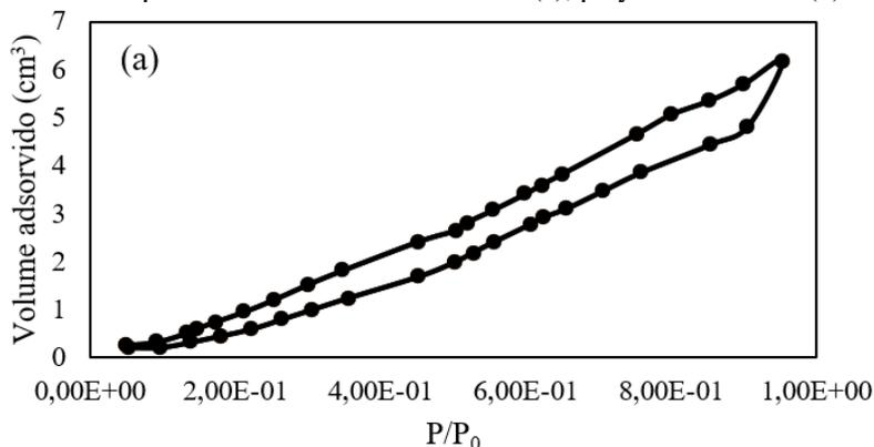
The profiles of the nitrogen adsorption and desorption isotherms presented by the three materials (Figure 3) do not correspond to any standard defined by the International Union of Pure and Applied Chemistry (IUPAC). The disordered syneresis of the isotherms suggests that the structure is disorganized and there is low affinity between the gas and the sample.
