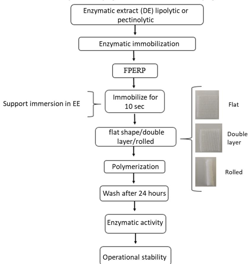
The immobilization of the enzymatic extracts in the flat form was performed by submerging the support in 3 mL of enzymatic extract, enough to cover the support, for about 10 s (maximum time stipulated by the manufacturer). Then, the support was removed and the end of the polymerization was waited, which occurs after 5 minutes, resulting in the hardening of the material.
