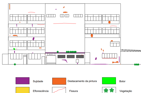
Figure 8 - Front façade damage map
