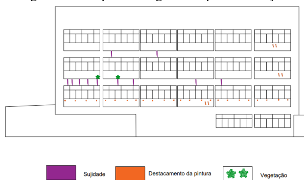
Figure 16 - Map of damage to the posterior façade
