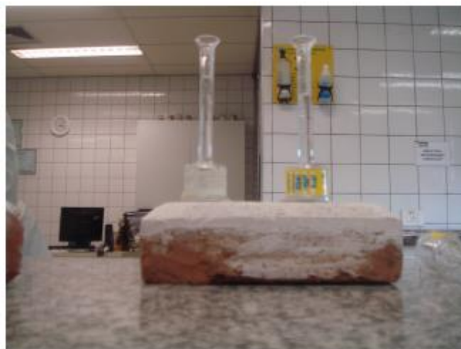
Figure 16: NBR 14992:2003 permeability test
