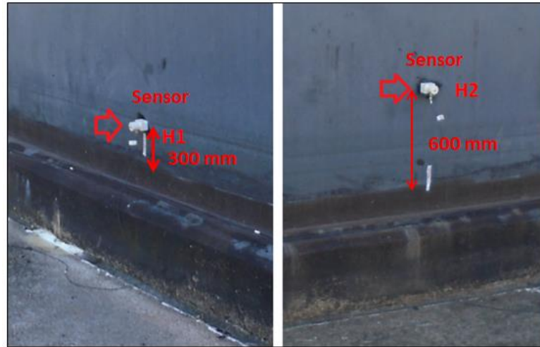
Figure 12 – Typical location where the sensors were installed odd (H1) and even (H2) positions
