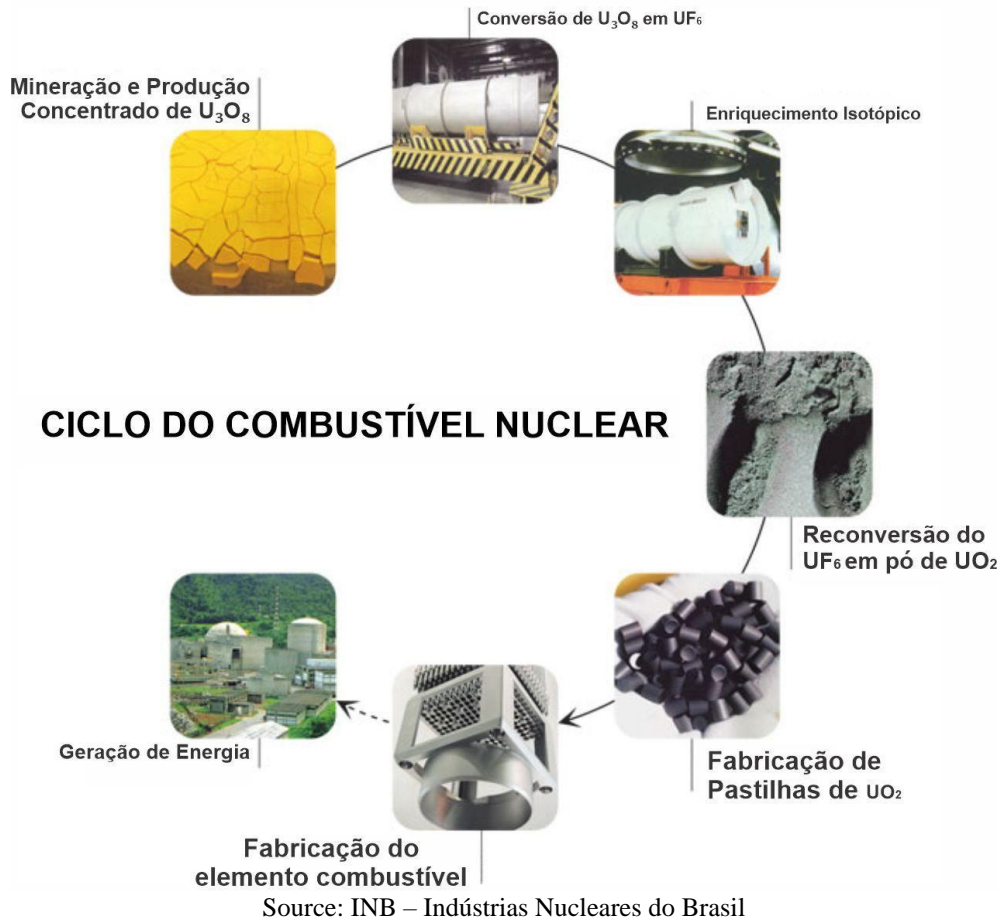
Figure 1 - Stages of the Nuclear Fuel Cycle
