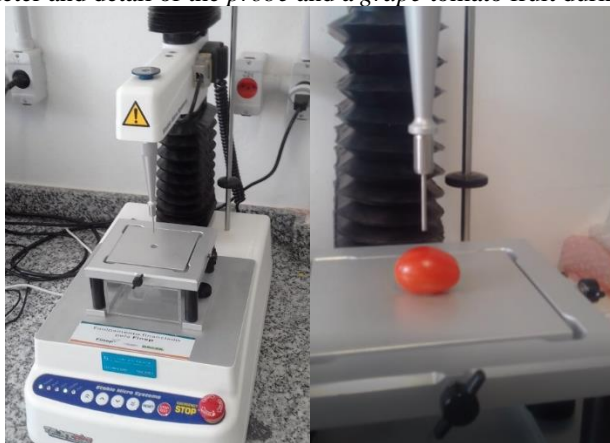
Figure 3: Texturometer and detail of the probe and a grape tomato fruit during firmness analysis.
