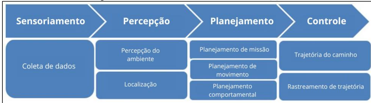
Fig. 2. Tasks in autonomous vehicles. Translated from [9].
