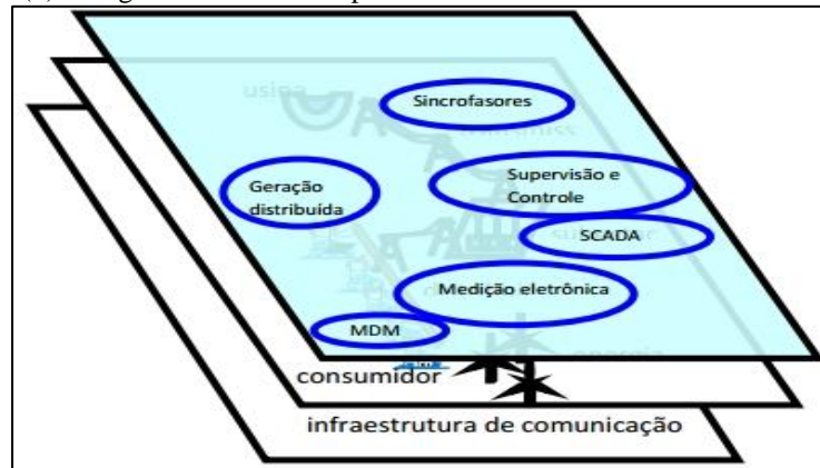
Figure (5) – Logical view of the supervision and measurement infrastructure [18].
