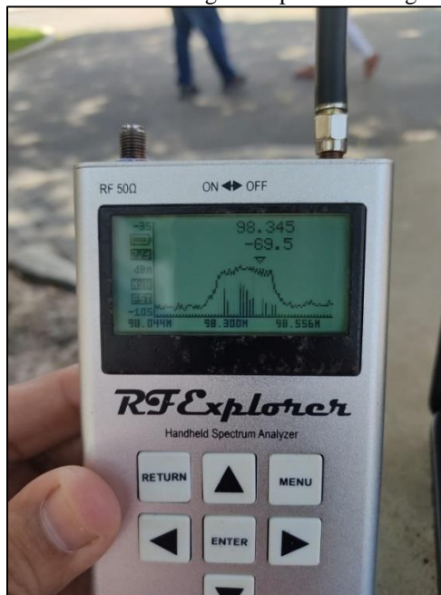
Figure 3. Measurement of the electromagnetic spectrum using the spectrum analyzer.
