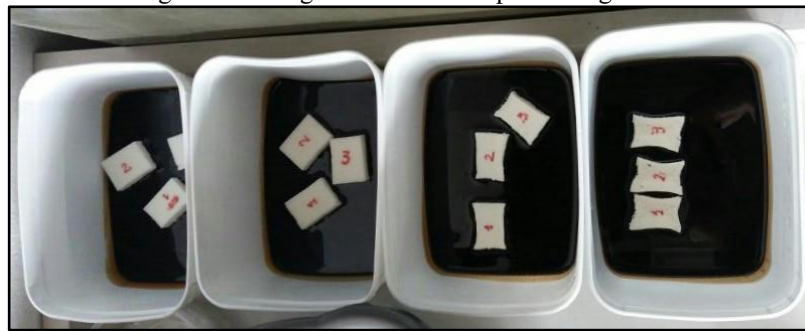
Figure 9. Arrangement of cut samples in engine oil.
