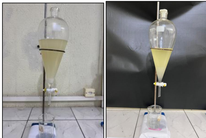
Figure 2. Process of decanting ethyl biodiesel from sunflower oil.
