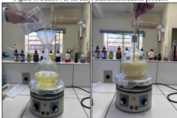
Figure 1. Sunflower oil ethyl transesterification process.
