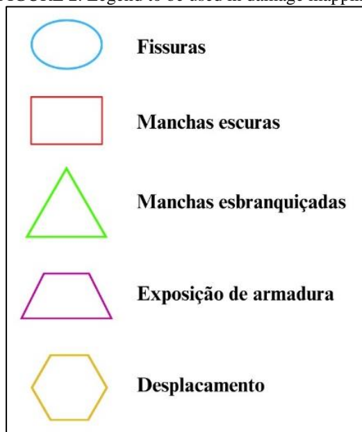
FIGURE 2. Legend to be used in damage mapping.
