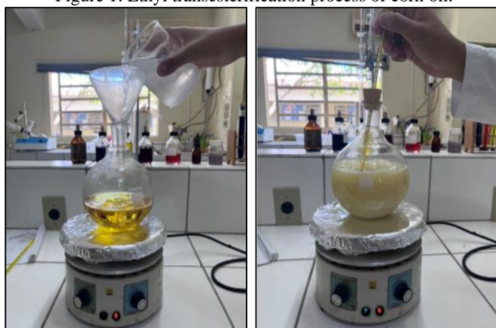
Figure 1. Ethyl transesterification process of corn oil.
