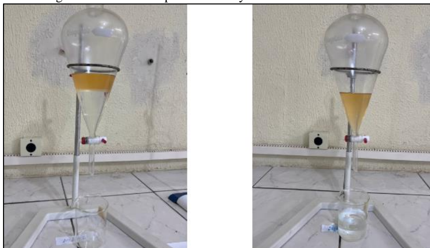
Figure 5. Decantation process of ethyl biolubricant from corn oil.
