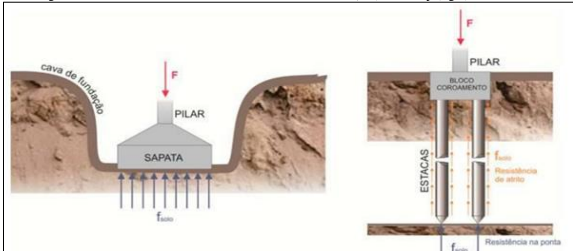
Figure 2 – Transmission of Loads to the Ground of Shallow (left) and Deep (right) Foundations.
