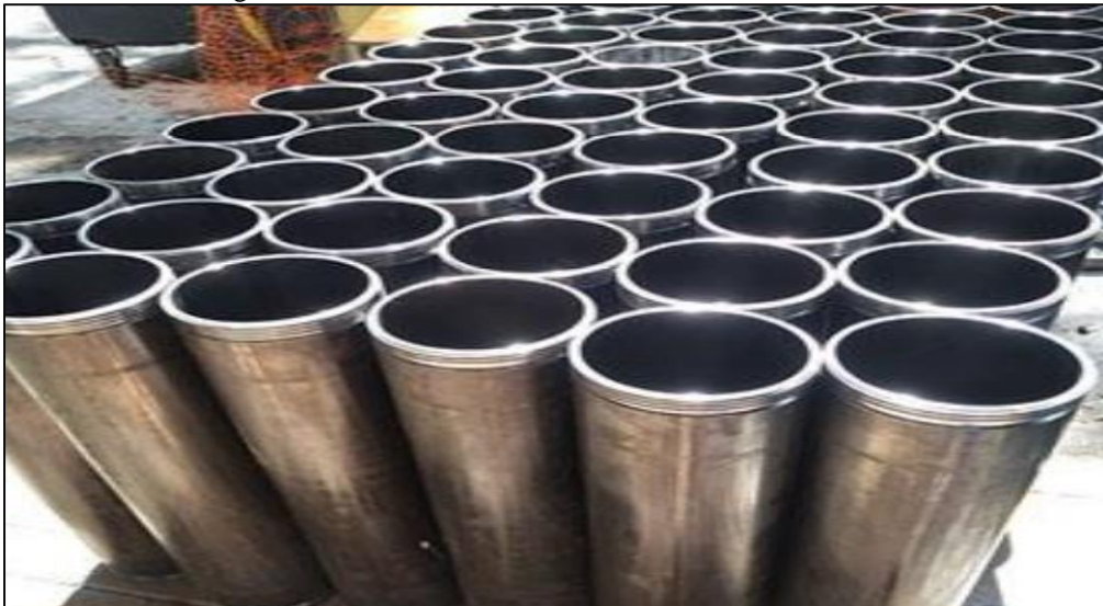
Figure 13 – Elements of the Metal Piles of 75cm Diameter.
