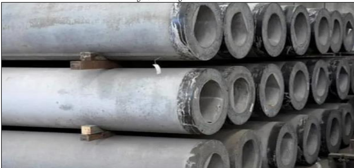
Figure 10 – Mega Precast Pile.
