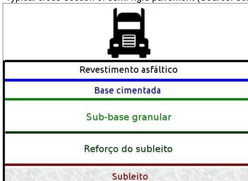
Figure 1.5 – Typical cross-section of semi-rigid pavement (Source: ecivilnet.com).
