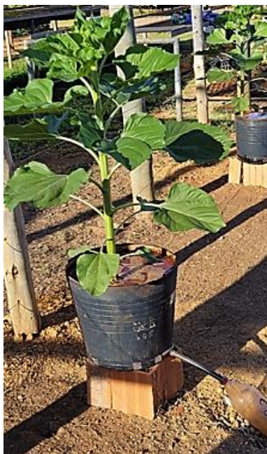
Figure 1 - Drainage lysimeter (a) and EVAPO software layout (b).
