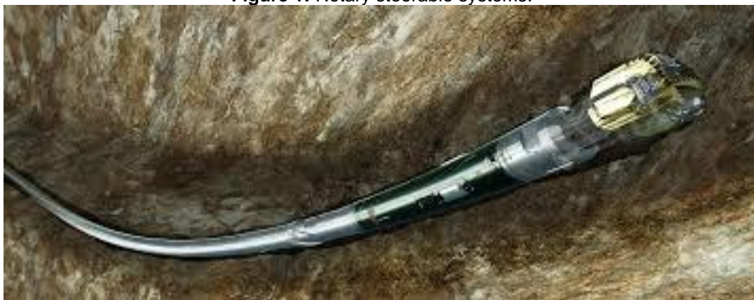
Figure 1: Rotary steerable systems.
