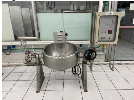
Figure 2 – Pilot Plant for Cheese Elaboration
