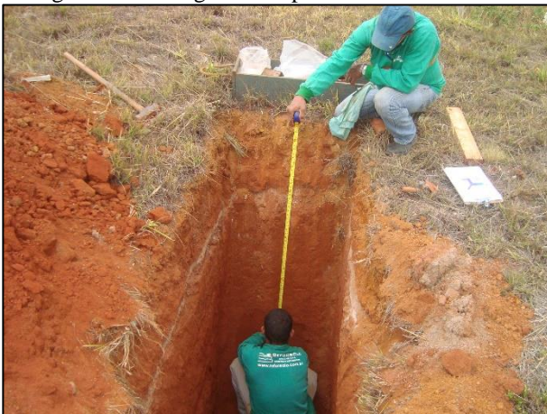
Figure 8. Inspection trench for carrying out “in situ” testing and collecting soil samples.
