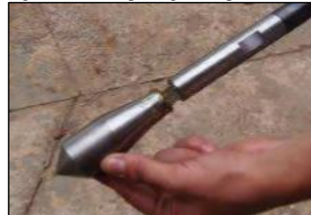
Figure 2. DPL tip for ground penetration.
