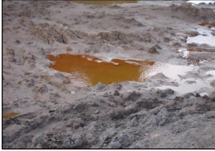
Figure 6. Existence of soft soil in section 1.
