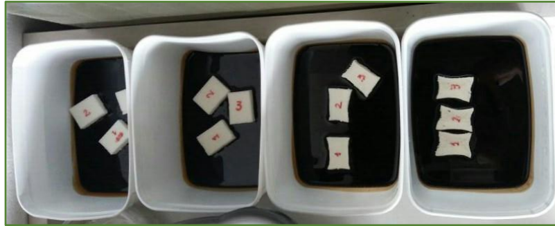
Figure 9. Arrangement of cut samples in engine oil.
