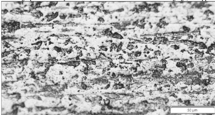
Figure 9 – Micrograph of the alloy submitted to solubilization and 0.5 h of aging (20x approximation).
