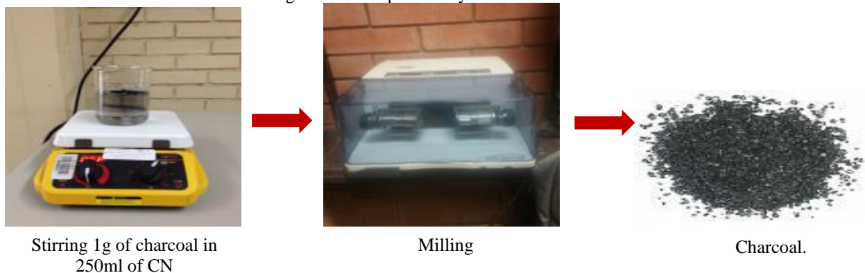
Figure 2: Adsorption of cyanide with carbon.
