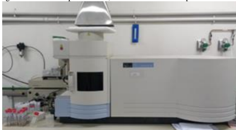
Figure 7: ICP-OES spectrometer, PerkinElmer model Optima 4300 used.
