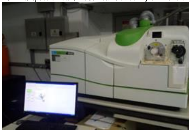
Figure 6: ICP-MS spectrometer, model NexIon 300 X from PerkinElmer used.
