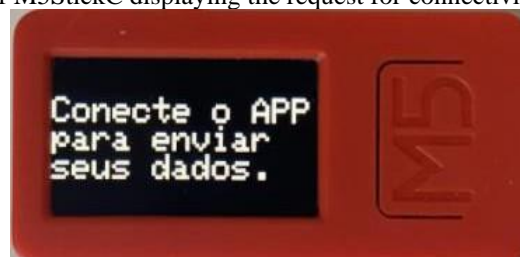
Figure 05: Image of M5StickC displaying the request for connectivity to the Application.
